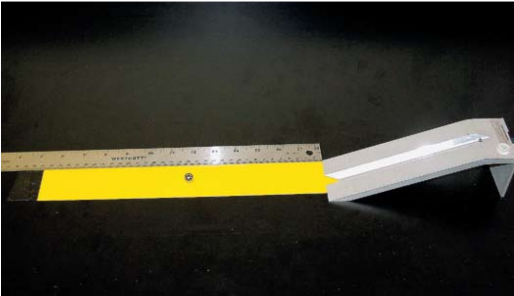
Figure 2. Rolling ball test apparatus and specimen showing distance of roll that is measured.
