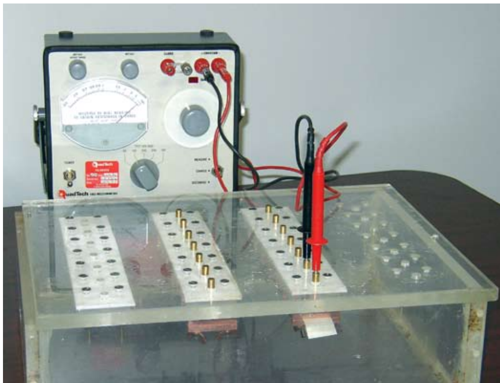
Figure 2. An arrangement for testing multiple tapes at the same time.
