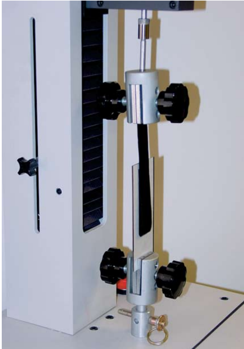
Figure 2. Adhesion to liner testing with tensile testing machine.
