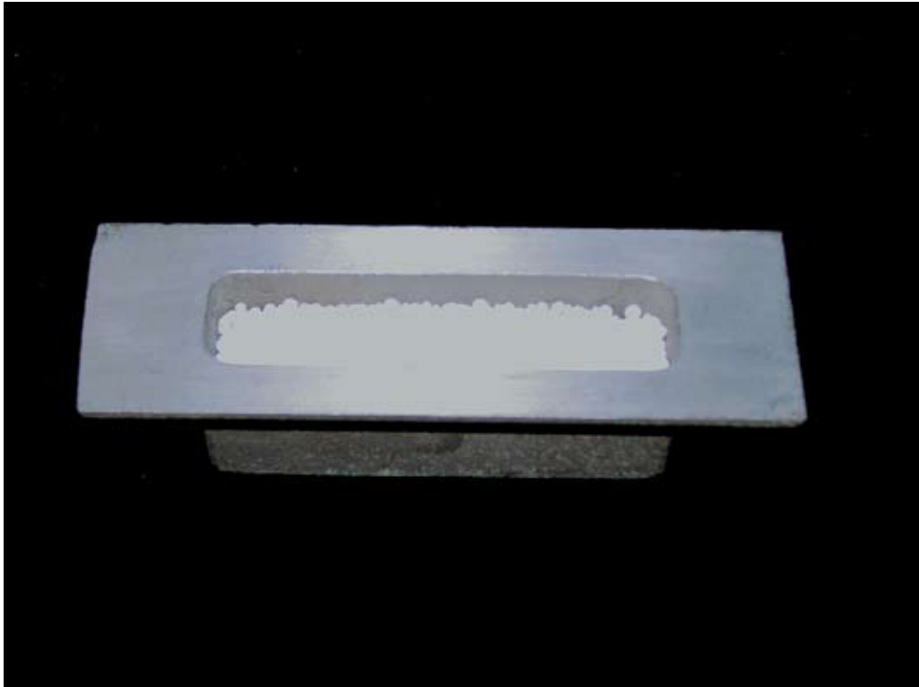
Figure 1. Water vapor cup filled with calcium chloride.
